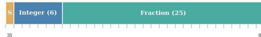
Fig. 3: Bit allocation of the 32-bit Q7.25 signed fixed-point word.
