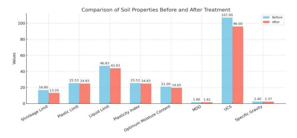
The results show a consistent deterioration in the properties of soil after leachate exposure.
