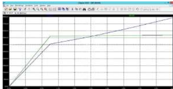
Fig7-DC analysis of conventional BGR
