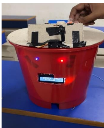
When the Dustbin is half full, it receives the garbage Fig 1.5
