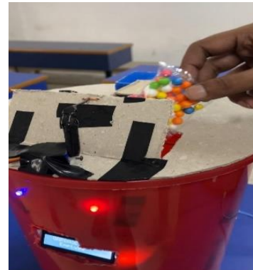
The Dustbin is receiving the Garbage, showing Dustbin is empty. Fig 1.4
