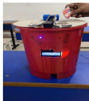
When the Dustbin is full, it does not allow to throw garbage Fig 1.6
