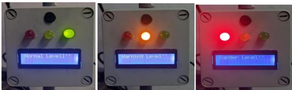
Figure 10: Display the conditions when water level detect the setting value
