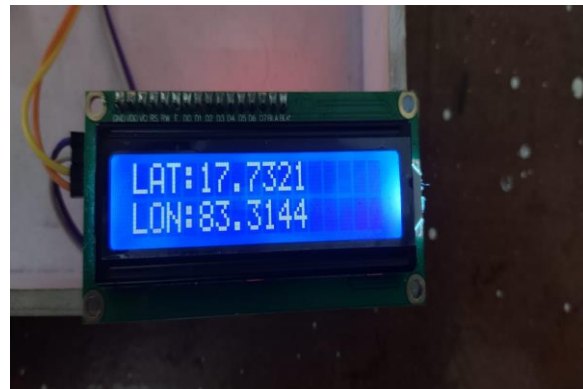
Fig: LCD display showing real-time GPS coordinates.
