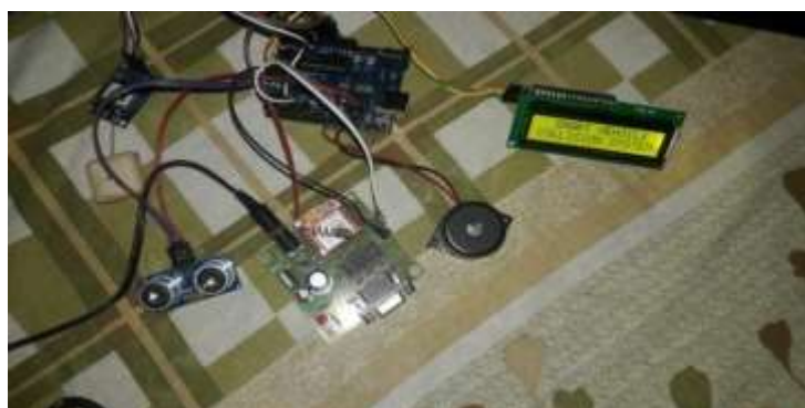
Fig.7. Hardware overview of smart vehicle accident collision detection system
