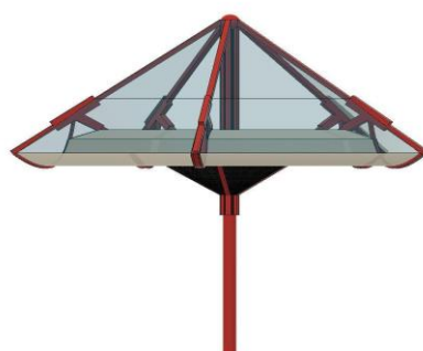
Figure 4: Side view of the 3D model of the umbrella desalinator
