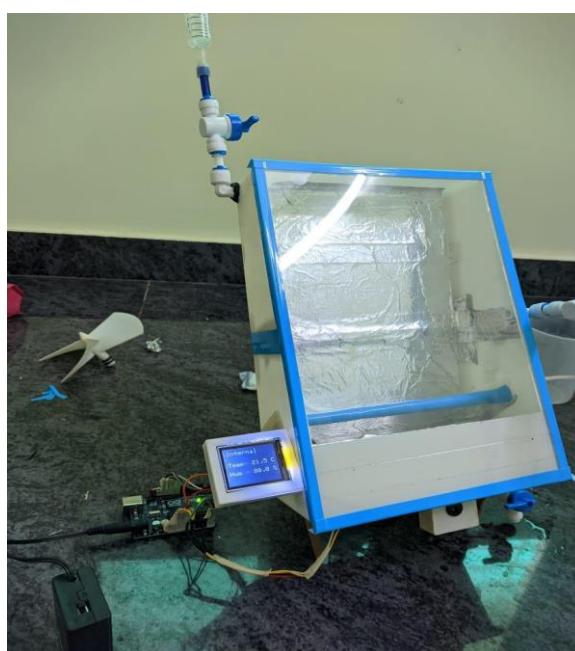
Figure 2: Prototype 1, with temperature and humidity sensor pictured.
