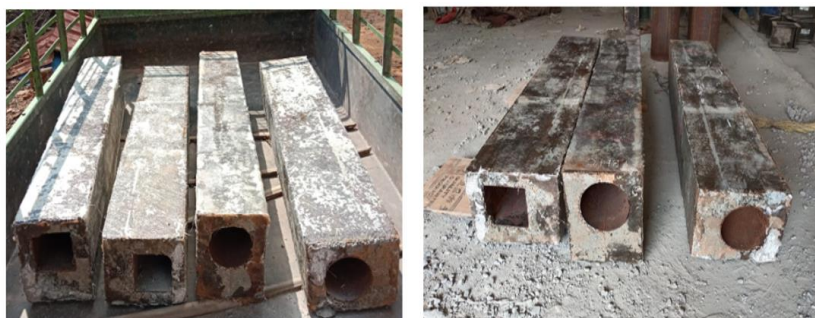
Fig 7. Steel-FRP- Concrete Hybrid Double Skin Tubular Specimens for Testing
