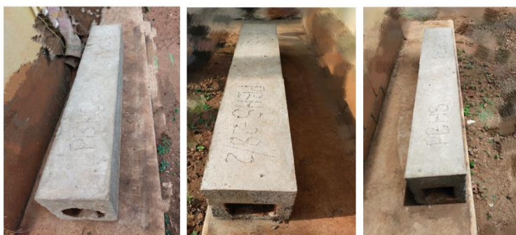
Fig 5. Specimens after Concreting
