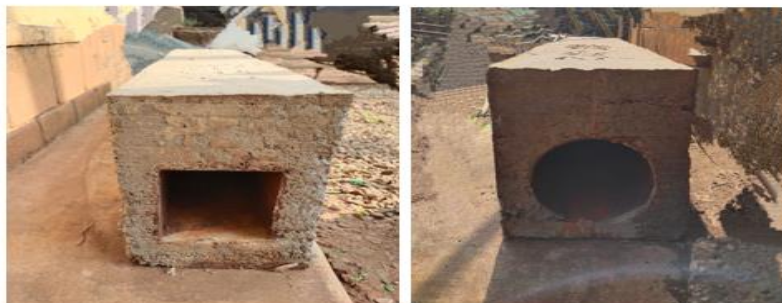
Fig 6. Cross sectional view of Square and Circular Specimens
