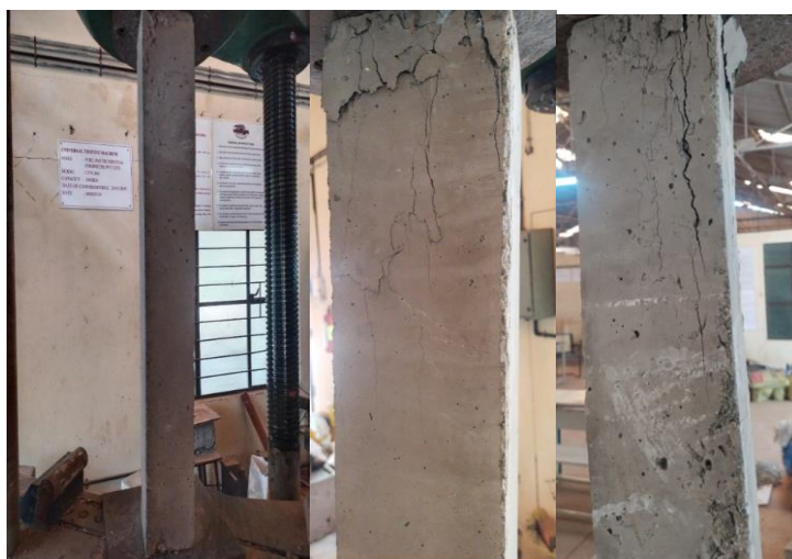
Fig 13: Different failure modes of RC column
