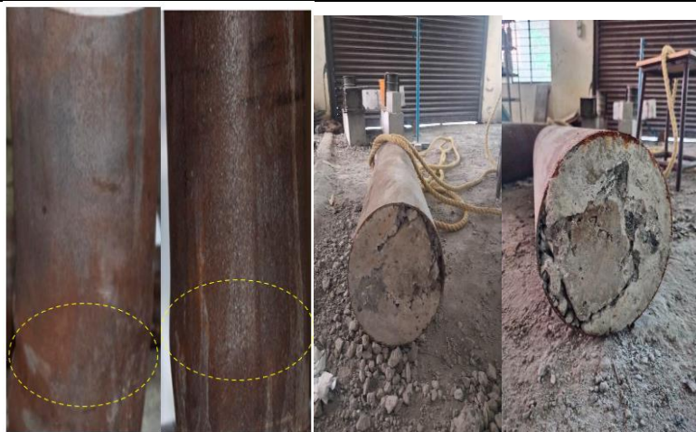
Fig 15: Different failure modes of strengthened columns
