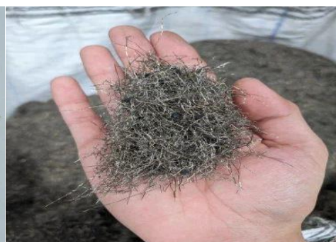
Fig 3: Recycled steel fibre
