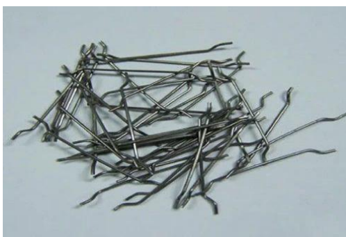
Fig 2: Industrial steel fibre
