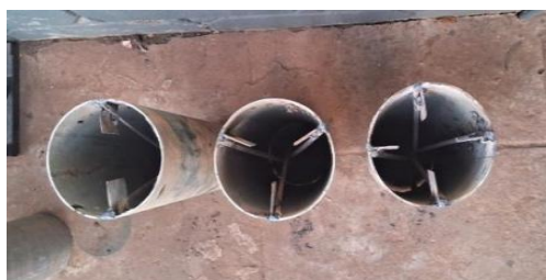
Fig. 1. Cross section of CFST column with steel bar stiffener
