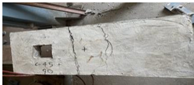
Fig 13. Crack pattern for S5 Slab
