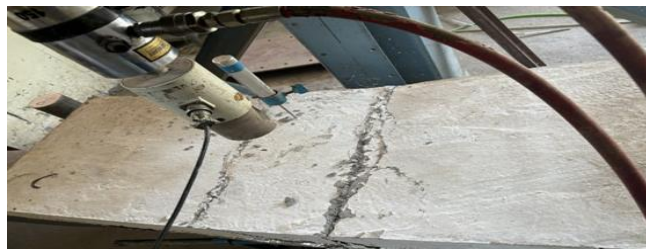
Fig 11. Crack Pattern in S1 Slab
