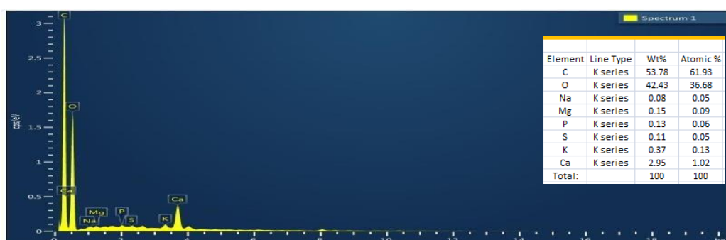
Figure 6: EDX analysis of banana peel after adsorption treatment
