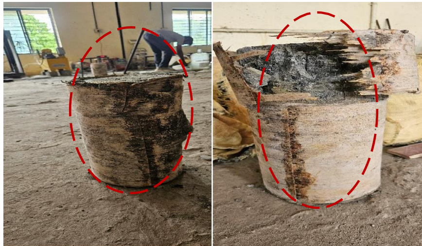
Fig 4. Typical failure modes of the BSTCC specimens.
