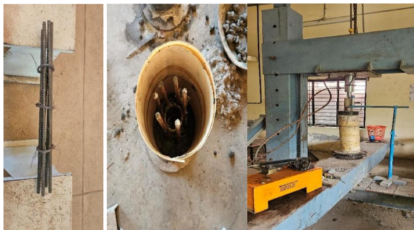
Fig 7. Strengthening of RC Column wrapping with Bamboo Sheet.
