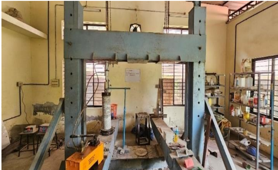
Fig 8. Loading Frame and Hydraulic Jack and Load Cell.
