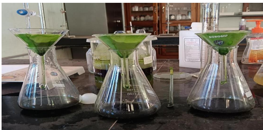
Fig .1. Neem powder, prepared neem extract using ethanol and neem extract filtration using filter paper
