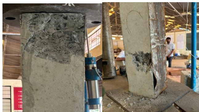
Fig. 7. Failure modes in ordinary PEC column with flat and corrugated web
