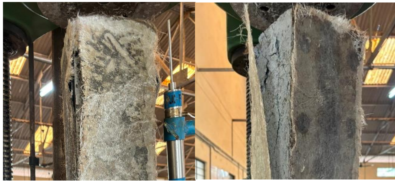
Fig. 8. Failure modes in GFRP wrapped PEC column with flat and corrugated web
